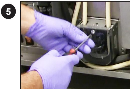
Remove cover with flathead screwdriver
