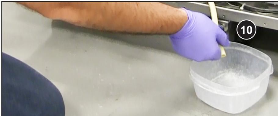
Let print material drain from hose into the drip container
