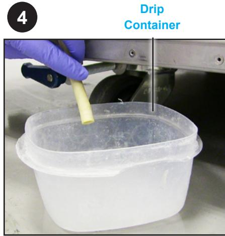
Place hose over drip container to catch any excess print material
